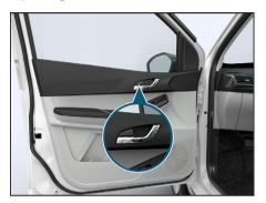
All doors can be opened from inside. To open, pull the door opening knob and then lever.
