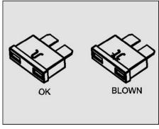
Remove the blown fuse by "fuse
