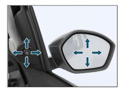
The switch to adjust the motorized mirrors is located on the driver's door. You can adjust the mirrors when the ignition switch is in the "ACC" or "ON" position.
