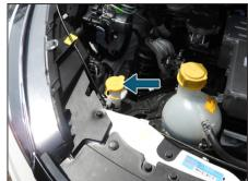
Measure the washer fluid in the tank. Fill with good quality windshield washer fluid (diluted with water) if the washer fluid level is low.
