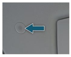
Mic is provided between the driver and codriver sun visors on roof.
