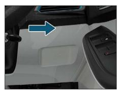
To remove the cover, gently pull the cover from bottom side such that the lugs get disengaged.
