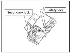
Secondary lock need to be opened and then safety lock to be pulled with suitable tool.  After successfully completion of service, press the secondary lock inside and safety lock to its original position.
