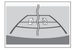
The distance guidelines will appear to be closer to the vehicle than the actual distance.
