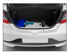
Use advance warning triangle to warn the approaching traffic in case of vehicle break-down or during emergency, where
