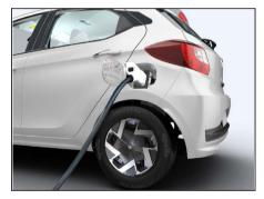
11. Charging Gun will be locked after switching on the DC charging station.
