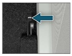
Pull the lever located at right side below near to driver seat to open the trunk lid.
