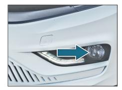
It turns 'ON' when the front fog lamp switch is pushed in with ignition 'ON' and position and parking / head lamp is 'ON'. An indicator on the switch will be illuminated when the front fog light is 'ON'.
