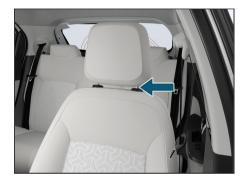
Adjust the head restraint so that it is as close to the head as possible and the center of the head restraint supports the back of the head at eye level. This will reduce the risk for injury to the head and neck in the event of an accident or similar situation.
